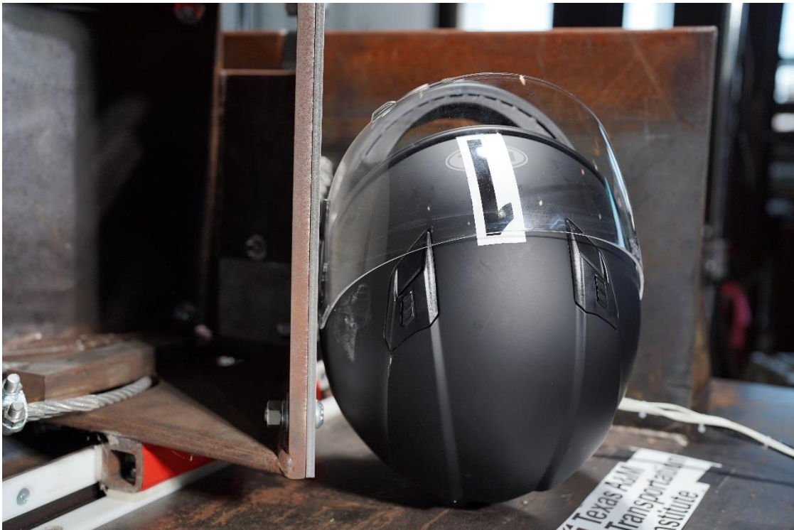
Figure 3.2. Test Apparatus at Contact Point.
