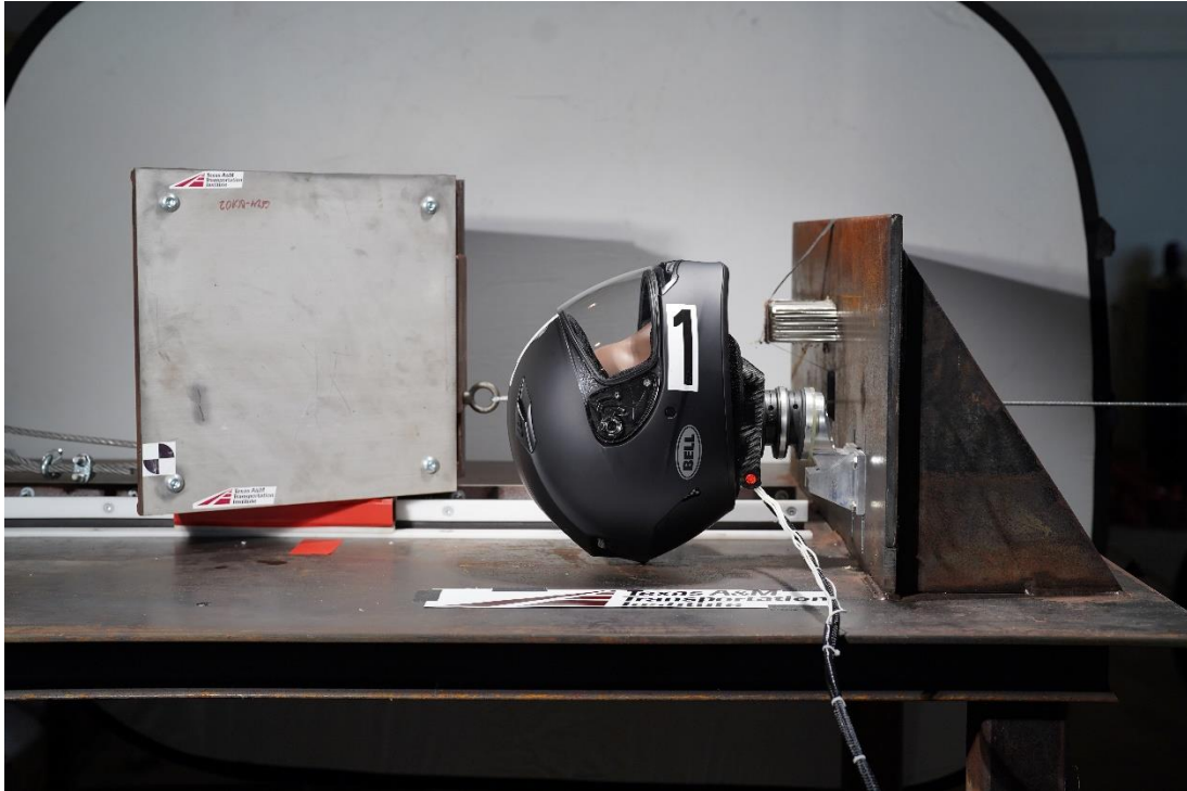
Figure 3.1. Test Apparatus and ATD Assembly with Motorcycle Helmet.
