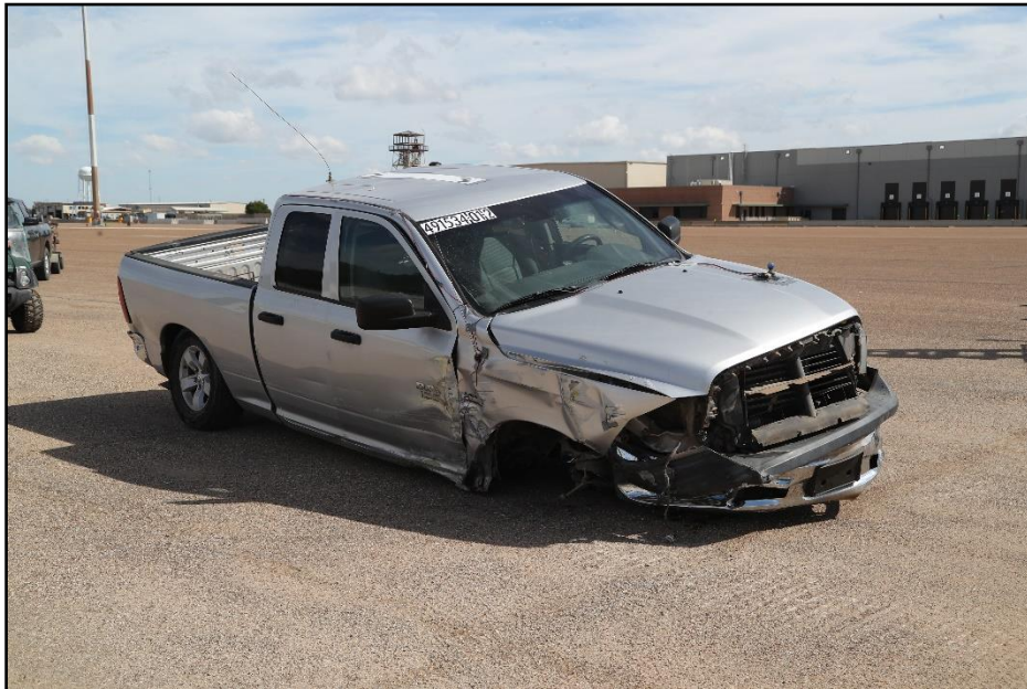
Figure 6.7. Impact Side of Test Vehicle after Test 491534-01-2.
