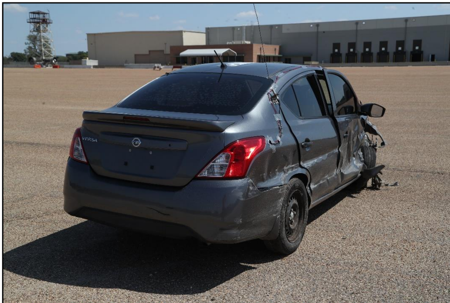
Figure 5.8. Rear Impact Side of Test Vehicle after Test 491534-01-1.
