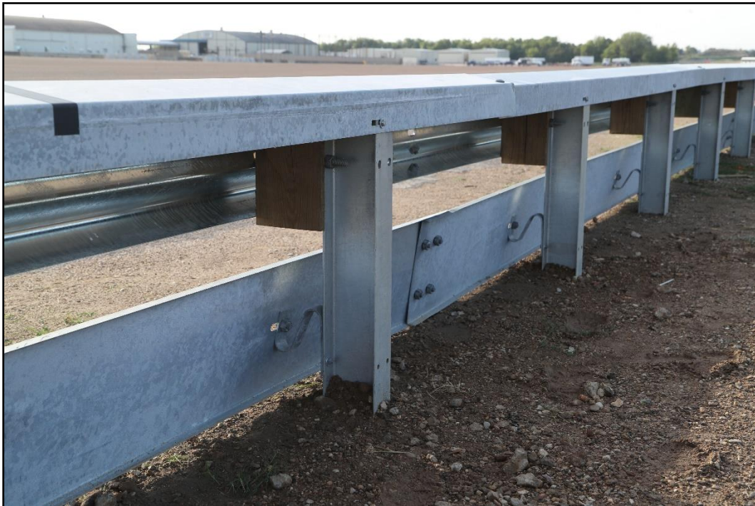
Figure 2.5. Oblique Field-Side View of Enhanced Motorcycle MGS prior to Testing.
