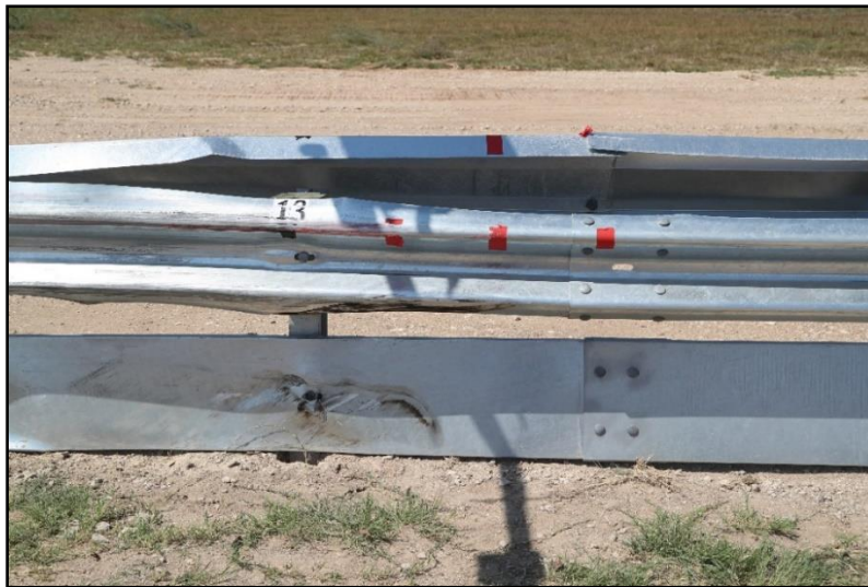
Figure 5.5. Enhanced Motorcycle MGS at Impact Location after Test 491534-01-1.
