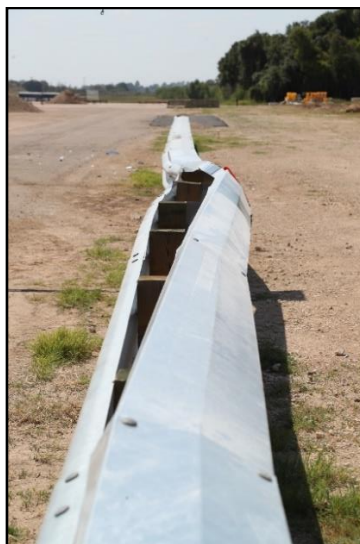
Figure 5.6. Downstream View of Enhanced Motorcycle MGS after Test 491534-01-1.
