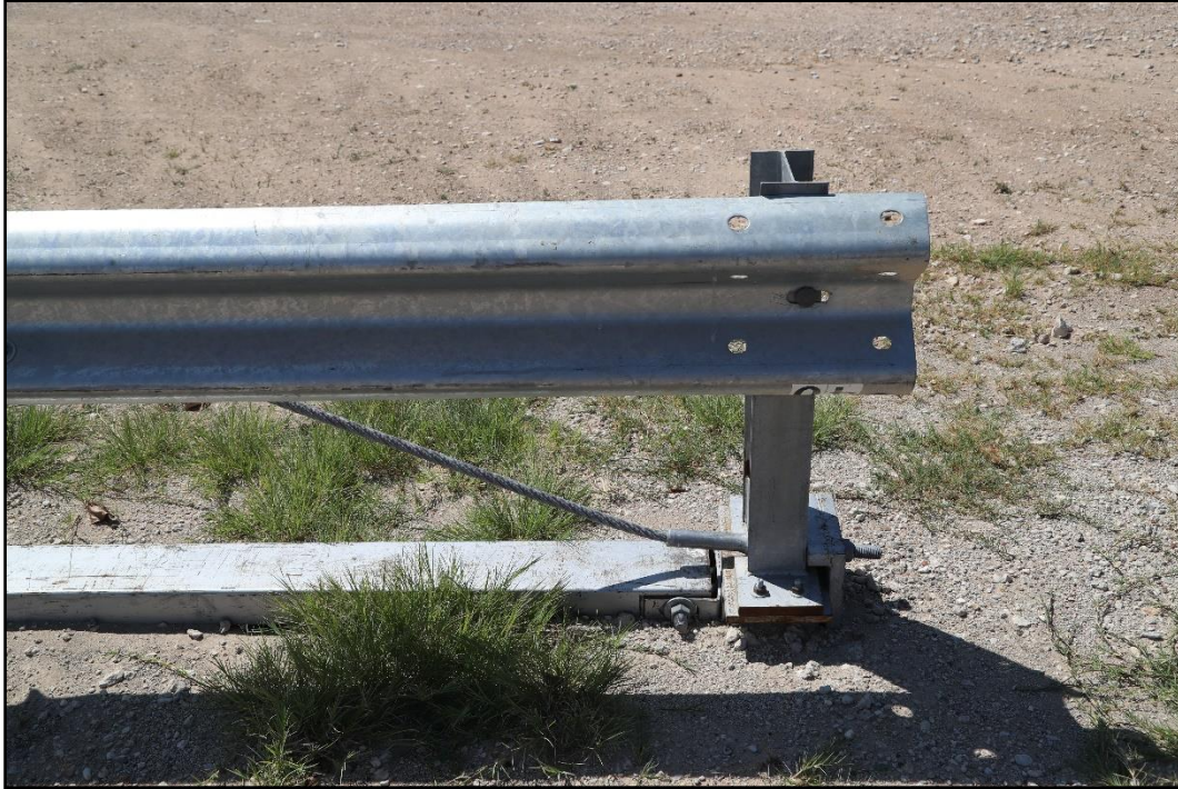
Figure 2.6. Focus on Post 1 without Rub Rail of the Enhanced Motorcycle MGS prior to Testing.
