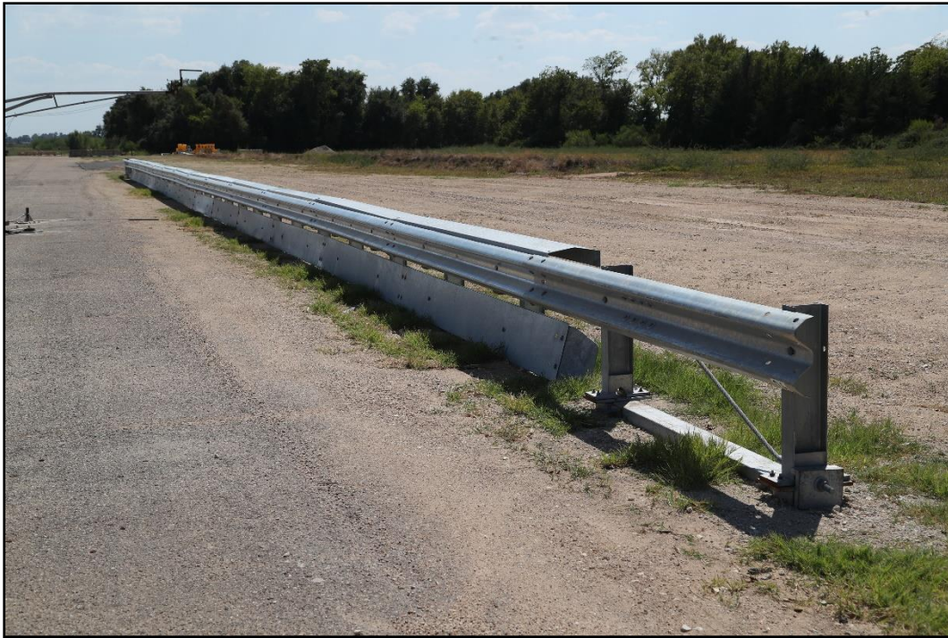
Figure 2.2. Overall View of the Enhanced Motorcycle MGS prior to Testing.
