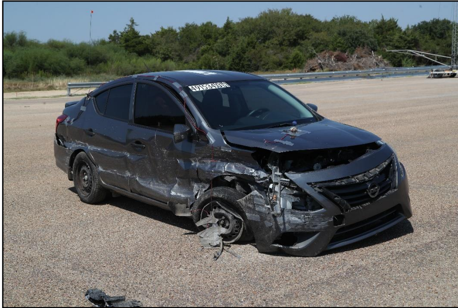
Figure 5.7. Impact Side of Test Vehicle after Test 491534-01-1.
