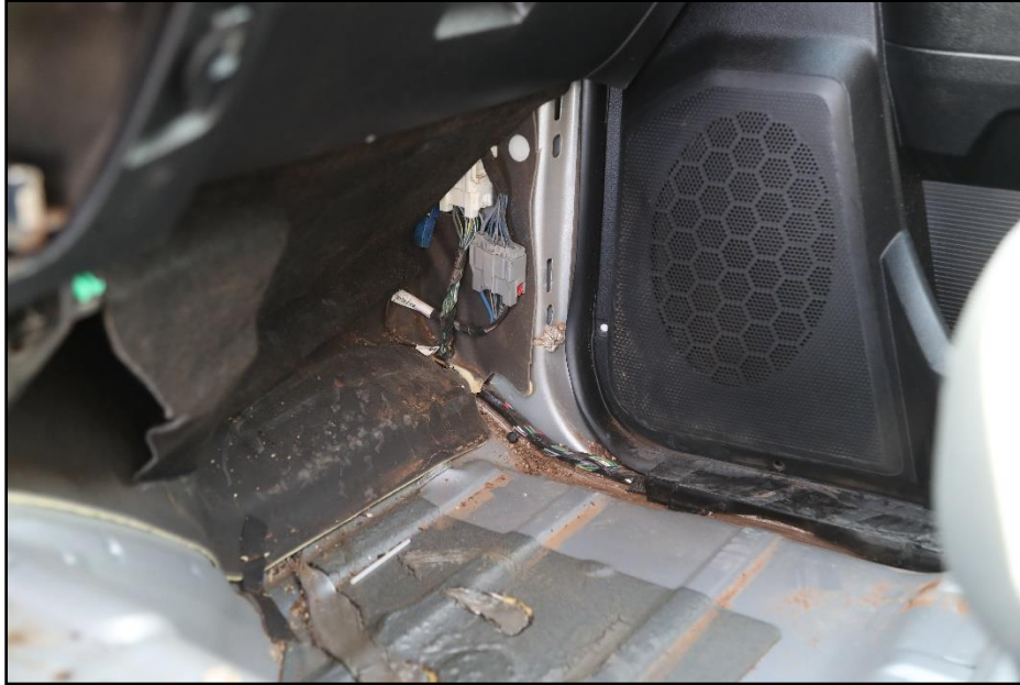
Figure 6.10. Interior of Test Vehicle on Impact Side after Test 491534-01-2.
