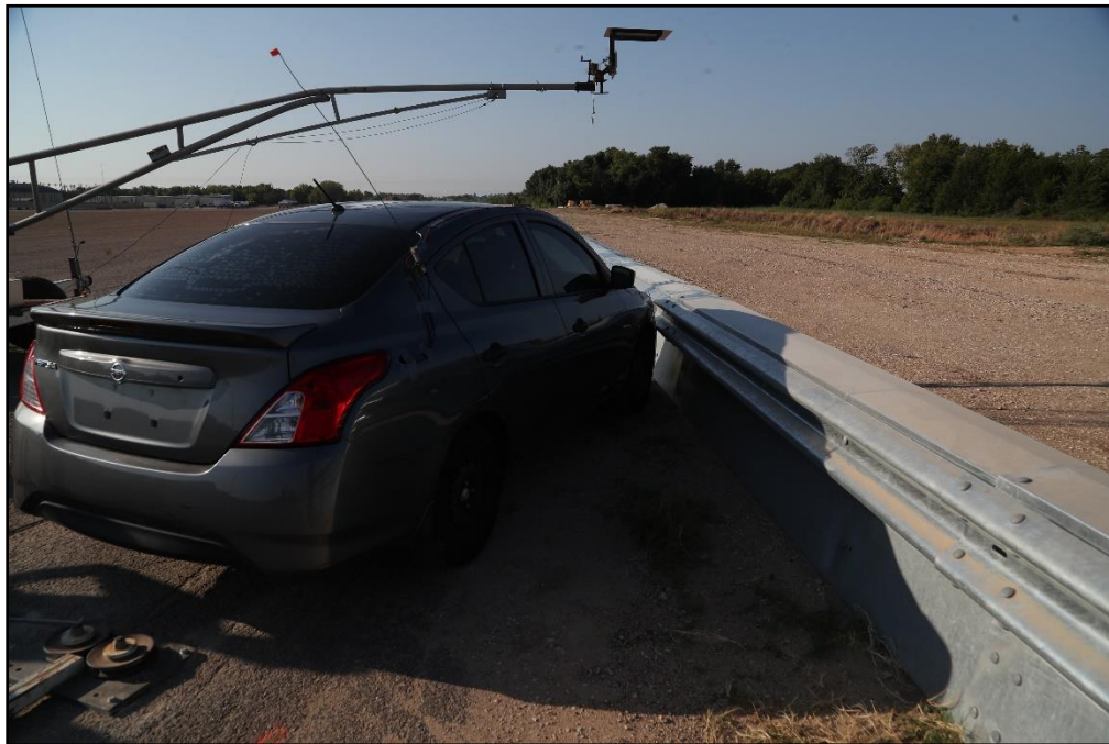
Figure 5.2. Enhanced Motorcycle MGS/Test Vehicle Impact Location for Test 491534-01-1.
