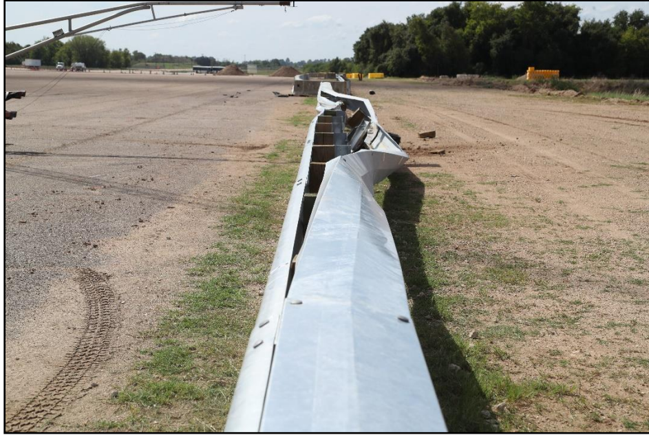
Figure 6.6. Downstream View of Enhanced Motorcycle MGS after Test 491534-01-2.
