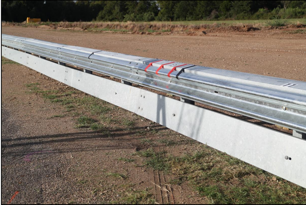
Figure 2.4. Enhanced Motorcycle MGS at Impact prior to Testing.
