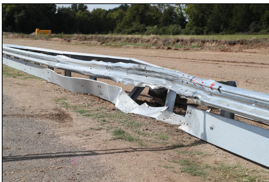
Figure 6.5. Enhanced Motorcycle MGS at Impact Location after Test 491534-01-2.
