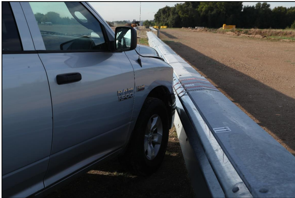
Figure 6.2. Enhanced Motorcycle MGS/Test Vehicle Impact Location for Test 491534-01-2.
